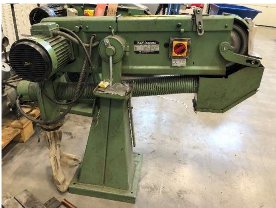
3. Bandslipmaskin KEF/Aldell BSH, slipbandet 75x2500 mm
