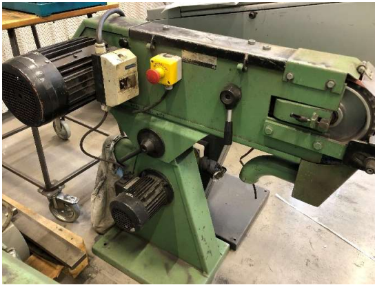
1. Bandslipmaskin KEF BSH 20-75, slipbandet 75x2000 mm
